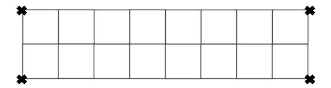
The four dissolved oxygen profile sampling stations shall be located at each corner of the net pen array. Dissolved oxygen will be measured at one meter of the water surface, at approximately half the depth of the pen, and within one meter of the bottom.
