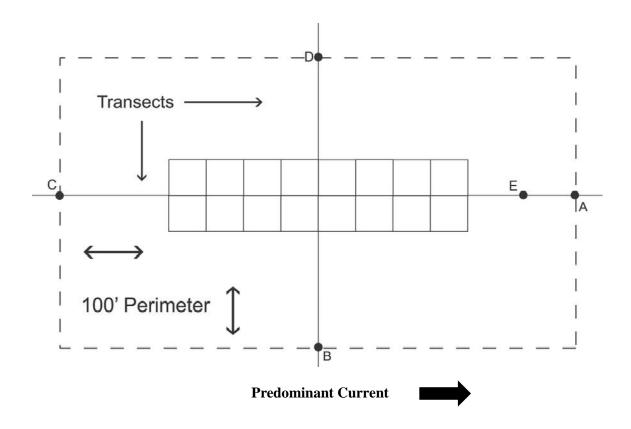
The five sediment sampling stations at the net pen facility shall be located along transects in line with the medial line of the long axis of the facility and in line with the short axis of the facility.
