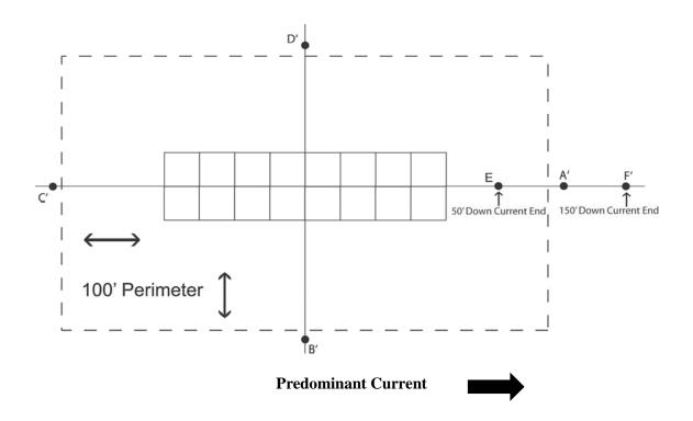
The six outside sediment sampling stations at the net pen facility shall be located along transects in line with the medial line of the long axis of the facility and in line with the short axis of the facility.
