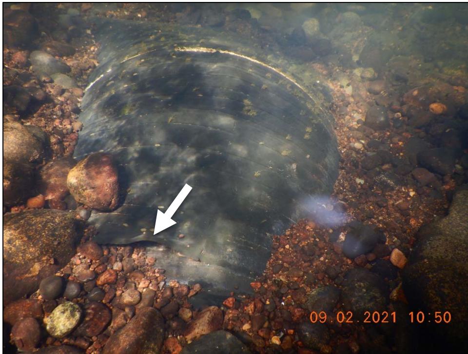
Photo 4: Minor Delamination and Tearing of Rubber (White Arrow) on Riser Check Valve #7
