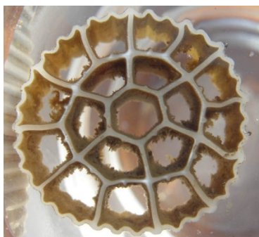
Figure 2-1 MBBR Carrier with Fixed Film Growth
