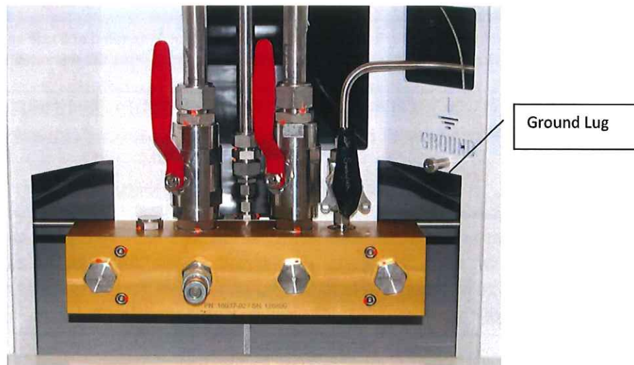
Figure 5: Grounding Lug
