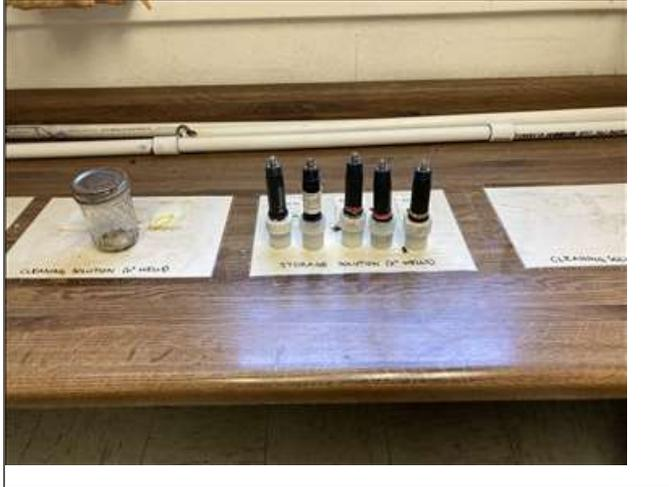
A photograph showing five pH probes lined up on a wooden table. To the left is a glass jar. Below the probes are two pieces of paper with handwritten labels: 'CLEANING SOLUTION (2" WELLS)' and 'STORAGE SOLUTION (2" WELLS)'. A long white pipe is visible in the background. | <p>pH probes used for 2" wells. Probes have salt around the rim of the cover and 3 did not have solution.</p> |
