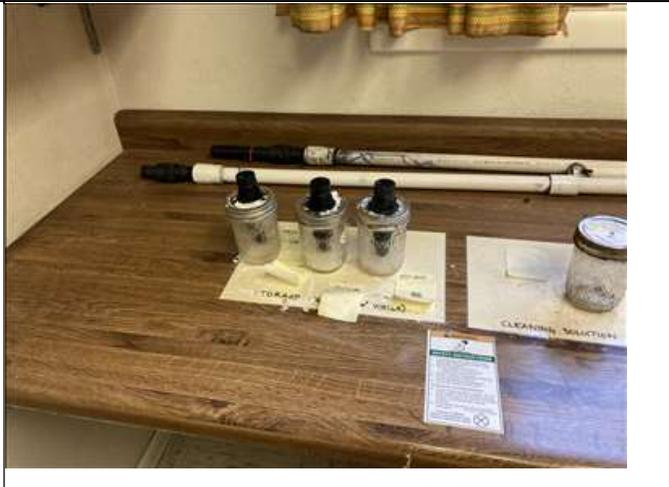
A photograph showing three pH probes and two glass jars on a wooden table. There are also some papers and a small white card on the table. A long white pipe is visible in the background.                                                                                     | <p>pH probes used for 6" wells. Jars did not have any storage solution.</p>                                   |
