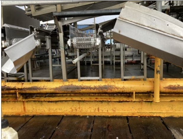
Photo 6. Fish sorting area, chutes that dump sorted fish into respective totes
