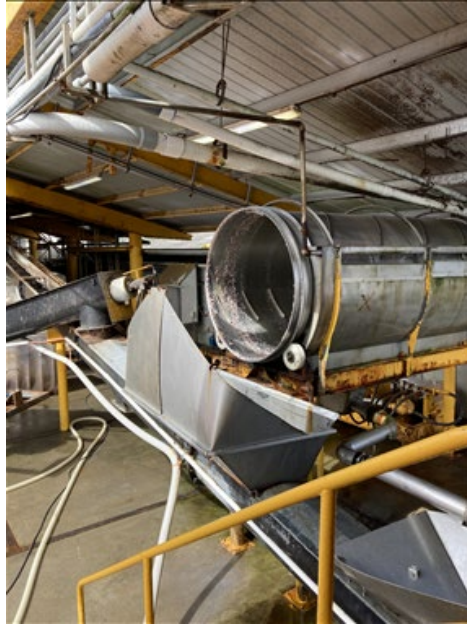
Photo 15. Second hydro-sieve that treats water from blue building.
