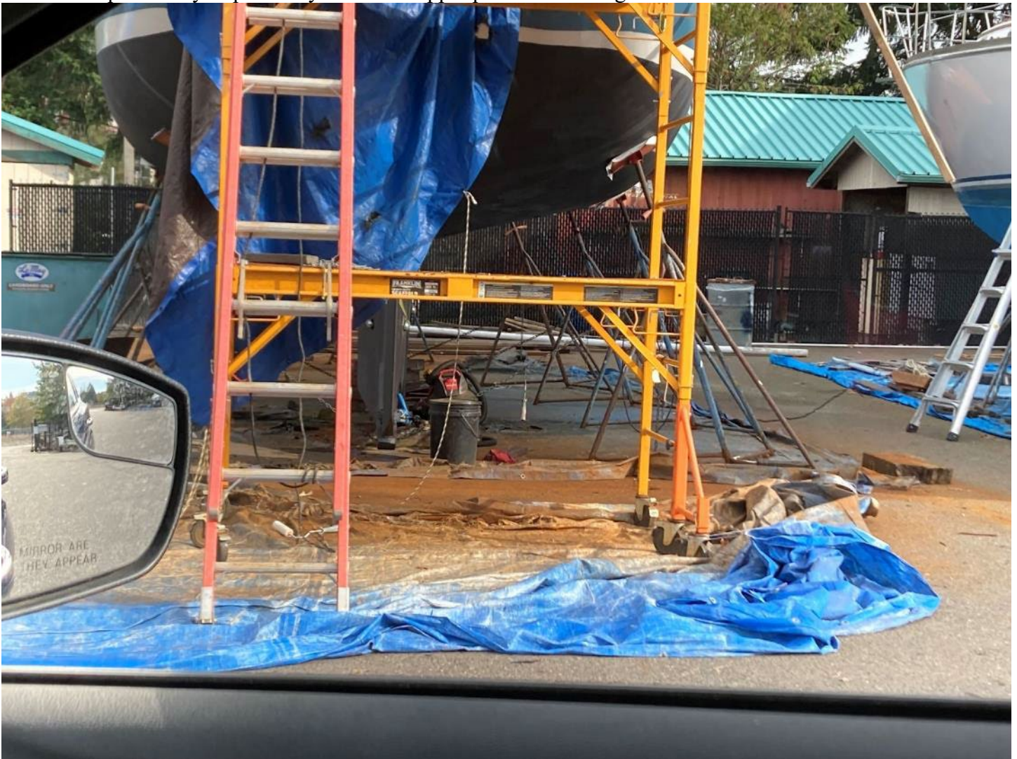
Photo 1: Opportunity for improved BMP maintenance. Rogue dust from grinding without a vacuum leads to stormwater potentially impacted by zinc and copper pollution. Facing east.
