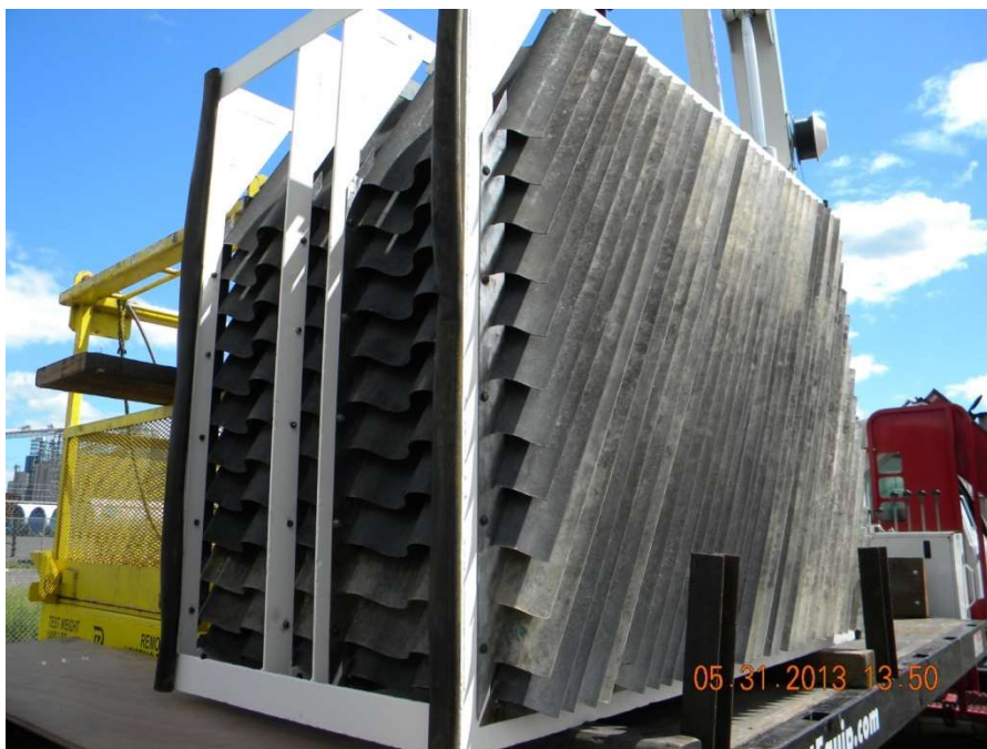
Figure 10.3: T-125 Plate Pack, Removed for Cleaning on 31 May 2013
