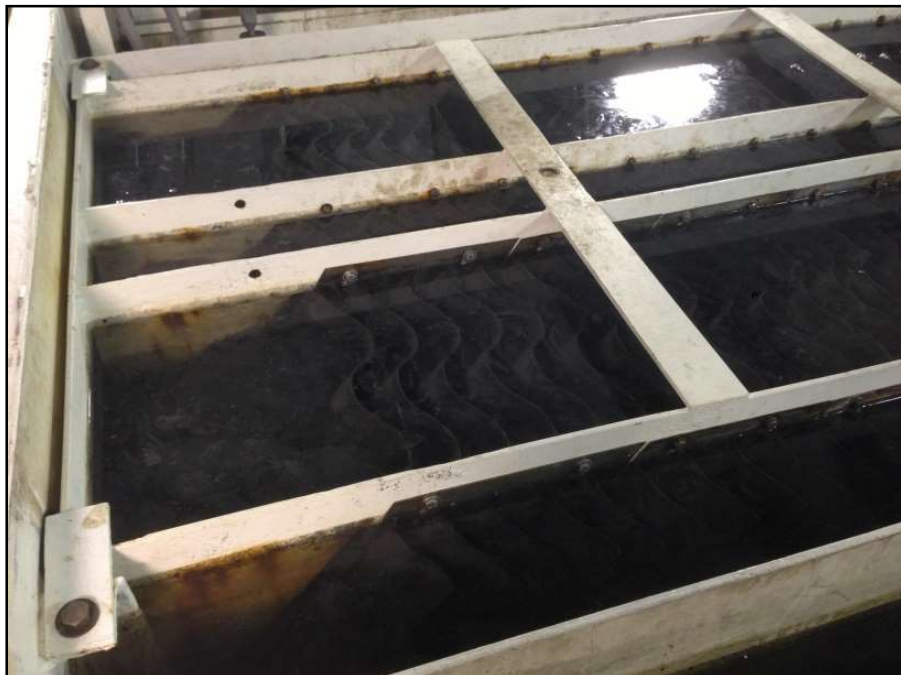
Figure 10.2: Top View of IPC T-125 with Plates Submerged
