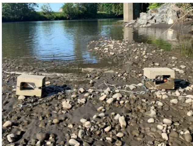
Figure 3. River thermistor deployment configuration
