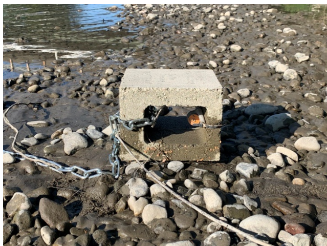
Figure 3. River thermistor deployment configuration
