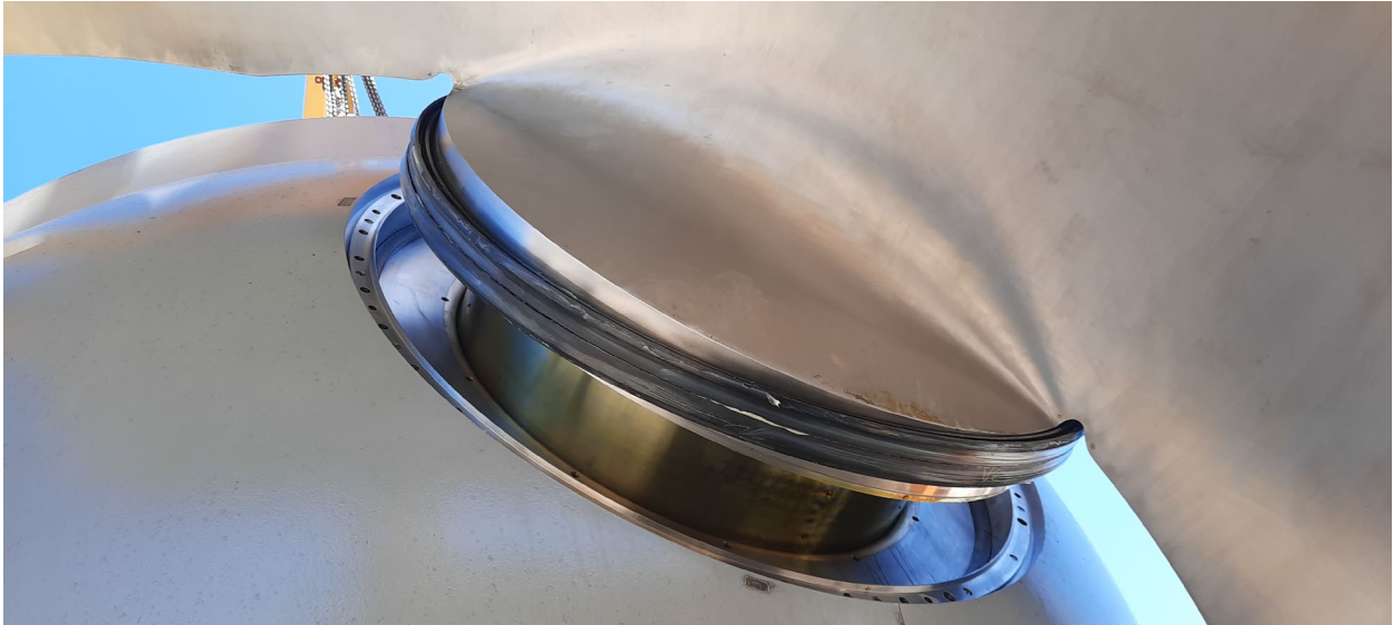
Figure 10. Kaplan Turbine Blade with Trunnion Seal during Assembly
