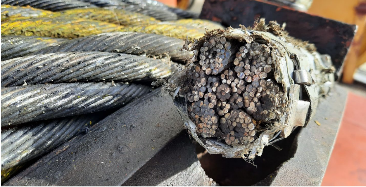
Figure 3. Wells Project Spillway Hoist Wire Rope with Strand Adjustment Visible
