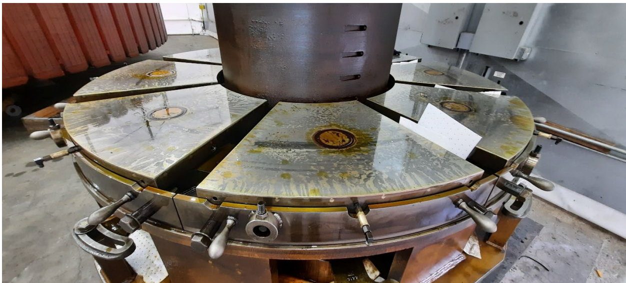
Figure 13. Wells Project Thrust Bearing Housing and Shoe Components after 55 Years of Service
