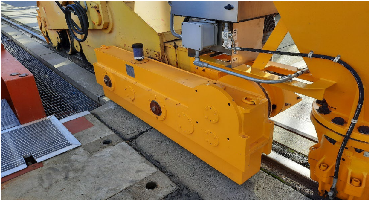
Figure 18. Wells Project Gantry Crane Driveline Gearbox
