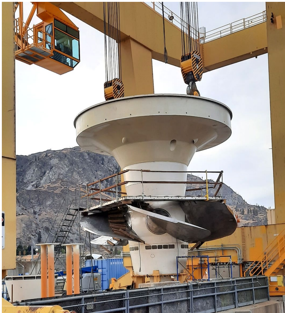
Figure 9. Wells Project Kaplan Turbine Assembly with Adjacent Headcovers ready for Installation
