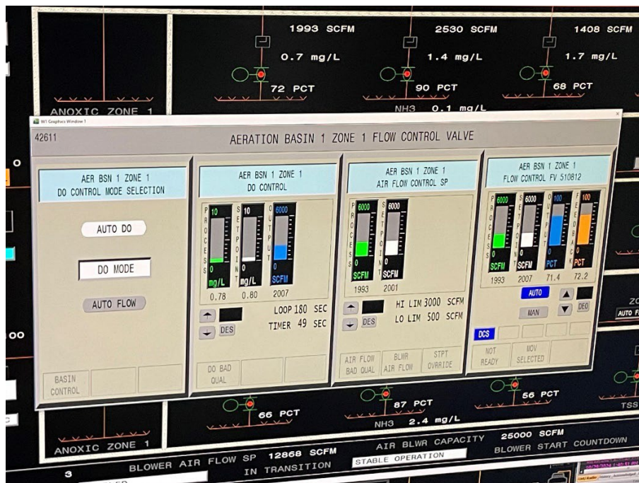
Photo 4 [IMG_1116] Description: Aeration Basin 1 DO Control Screen
