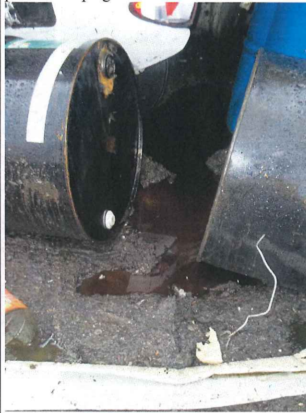
Photo 12 of 12: Sampling point 3 under the pile. There were drums not properly emptied prior to scraping.
