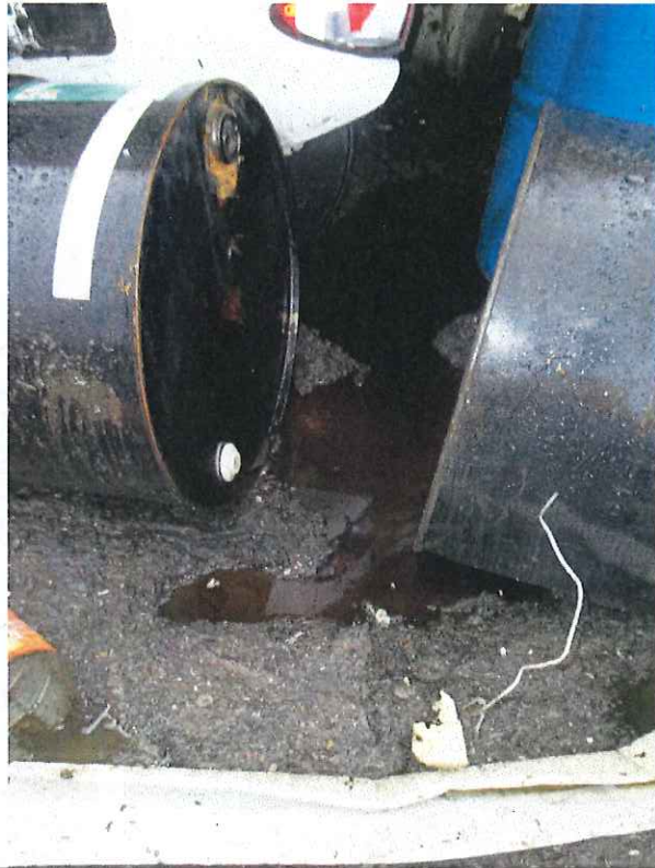
Photo 8 of 12: Open oil containers stored outside, no secondary containment and exposed to stormwater.
