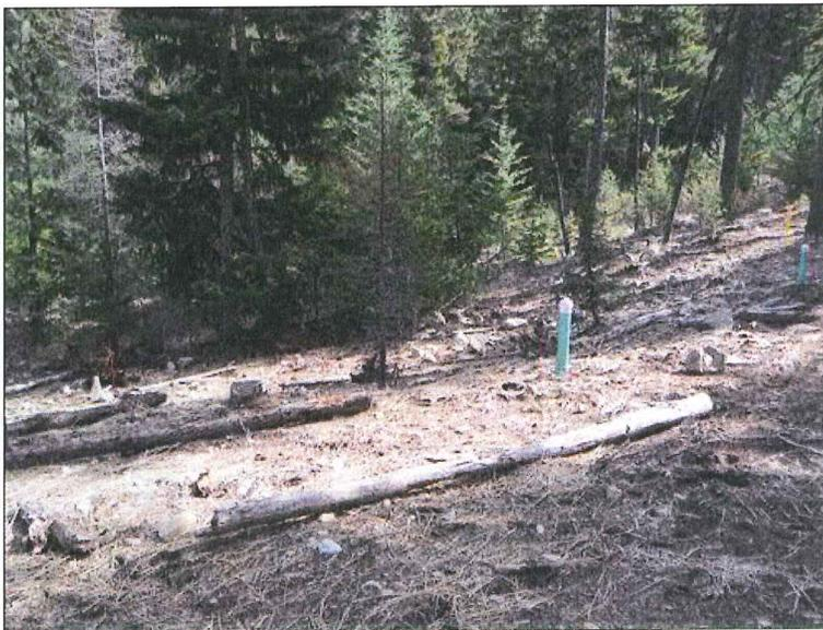
A photograph showing a wooded area with several observation ports (green pipes) and settlement stakes (yellow and blue) installed in the ground. A large log lies on the ground in the foreground. |
