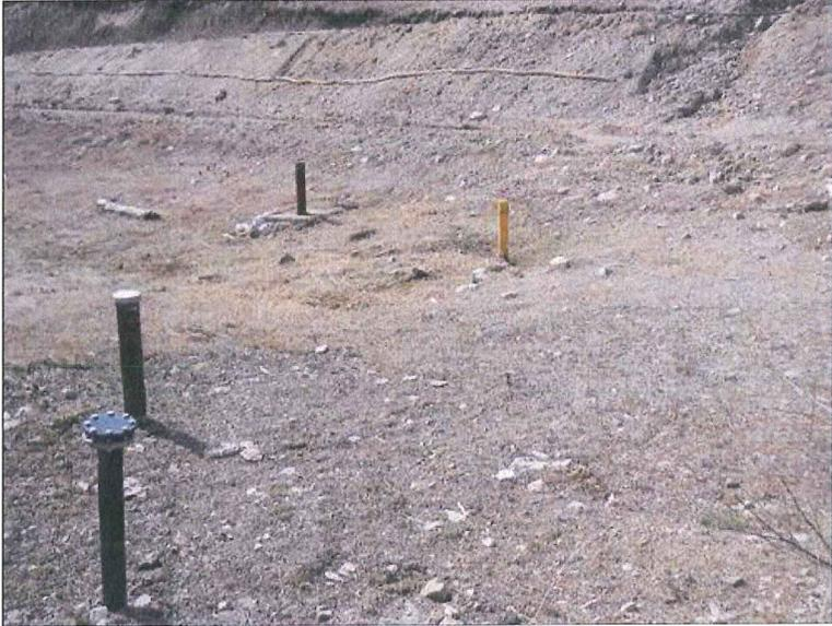
A photograph of a monitoring well KW1-A at the Key Mine site. The well has a yellow casing and is situated in a gravelly, open area. In the background, a large waste rock dump is visible. Other monitoring wells are also present in the area. |
