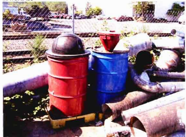
P5160040 DESCRIPTION: BARRELS OF HAZARDOUS MATERIALS KEPT ON SECONDARY CONTAINMENT FULL OF RAIN WATER
