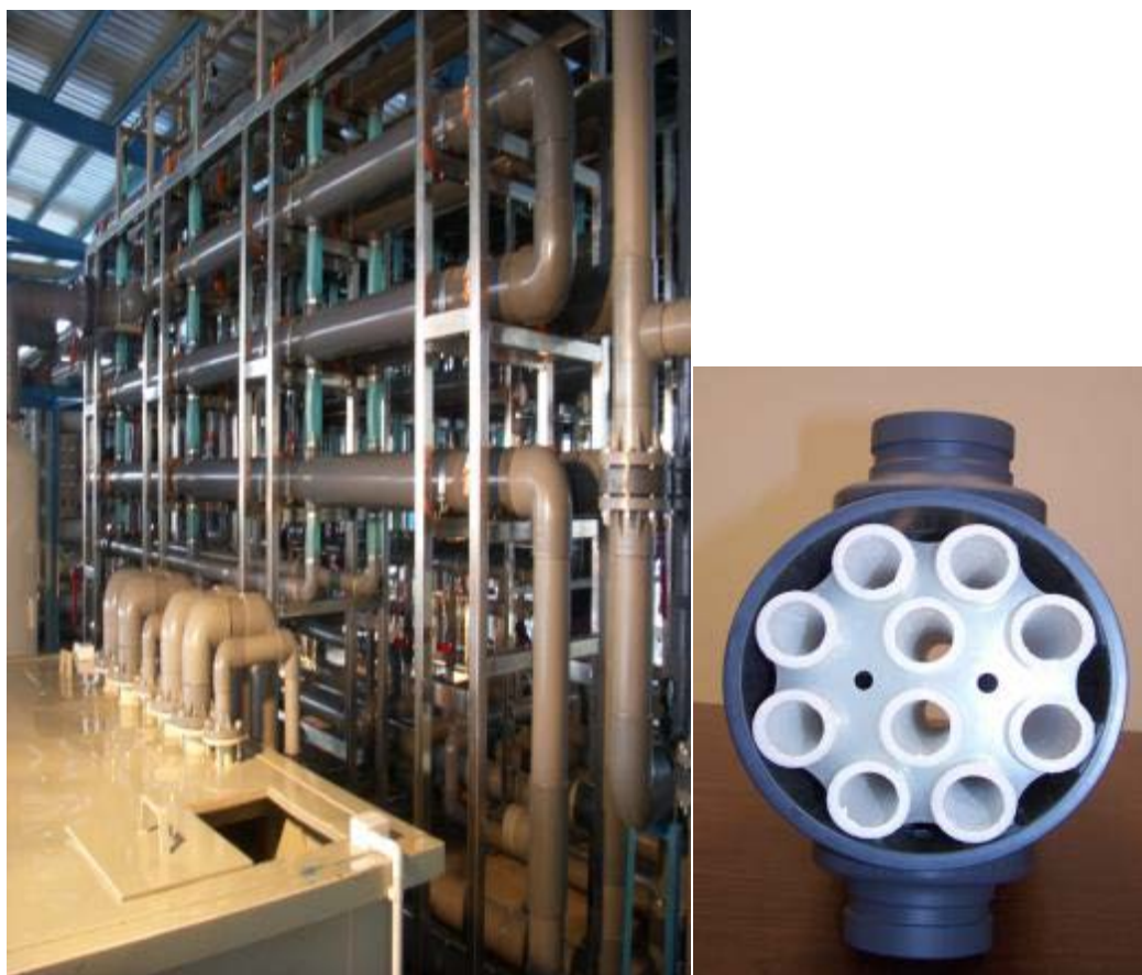
Figure 5-2. Duraflow MF system with tubular MF module
