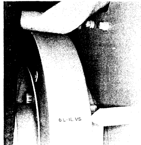
Fig. 2-59, (K21917). Valve set marks on vibration damper —KT/KTA38
