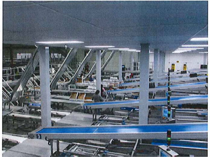
Cherries after cluster cutter to cameras and grading. Final packing before conveyed to shipping.
