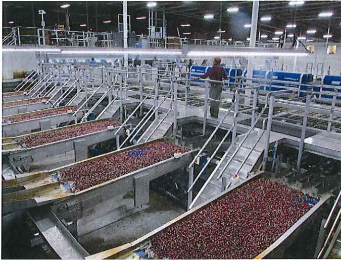
Cherries after cluster cutter to cameras and grading. Final packing before conveyed to shipping.
