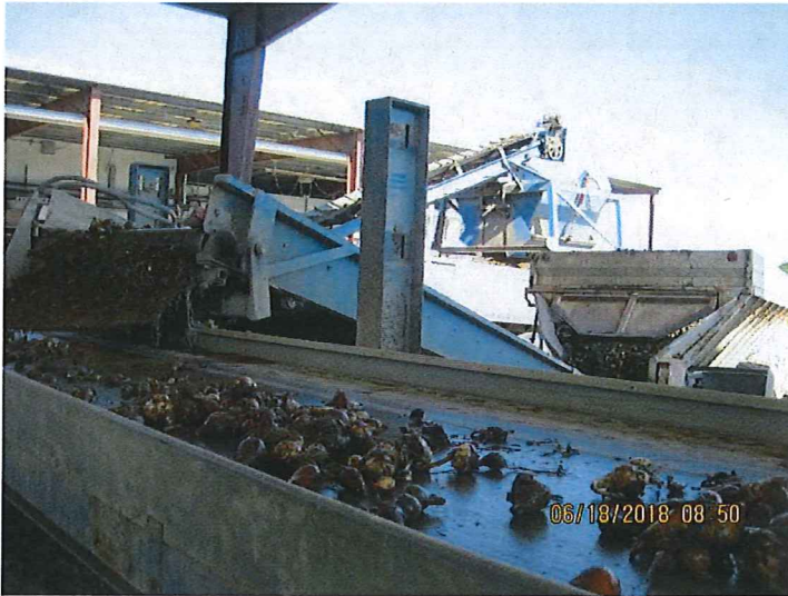
PHOTO 1 DESCRIPTION: FIELD WASHED BULBS HEADING TO ROTARY WASHER.
