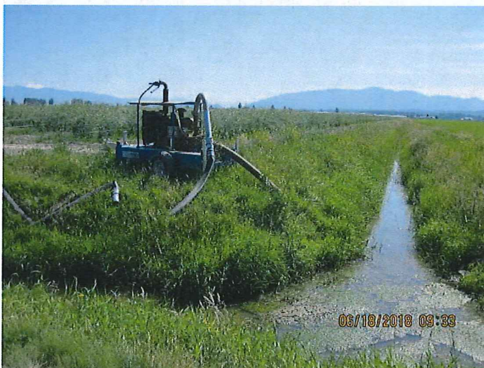
PHOTO 23 DESCRIPTION: LOCAL IRRIGATION PUMP SET TO WITHDRAW WATER FROM AGRICULTURAL DITCH.
