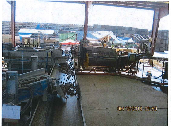
PHOTO 2 DESCRIPTION: ANOTHER VIEW OF CONVEYOR FROM TRUCKS. ROTARY WASHER IS IN THE CENTER REAR.
