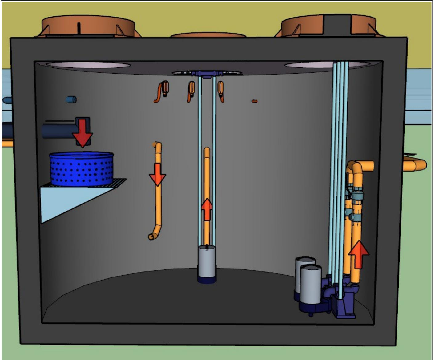
Wastewater enters the tank on the left and falls through the screen. Mixer pump in the center of the image with the mixer return to the left. Discharge pumps on the right.
