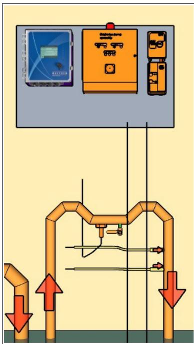
The mixer pump circulates water through a loop inside the building. This pH control loop contains, in order, a pH electrode, sample port, and two chemical addition ports. The mixer and chemical addition system will run any time the tank level is greater than 30%.
