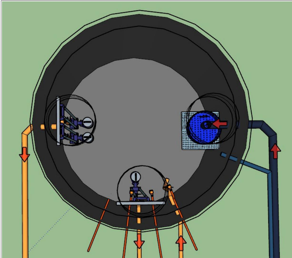
One mixer pump is visible on the bottom, with two discharge pumps on the left. The discharge pumps alternate with each pump cycle.
