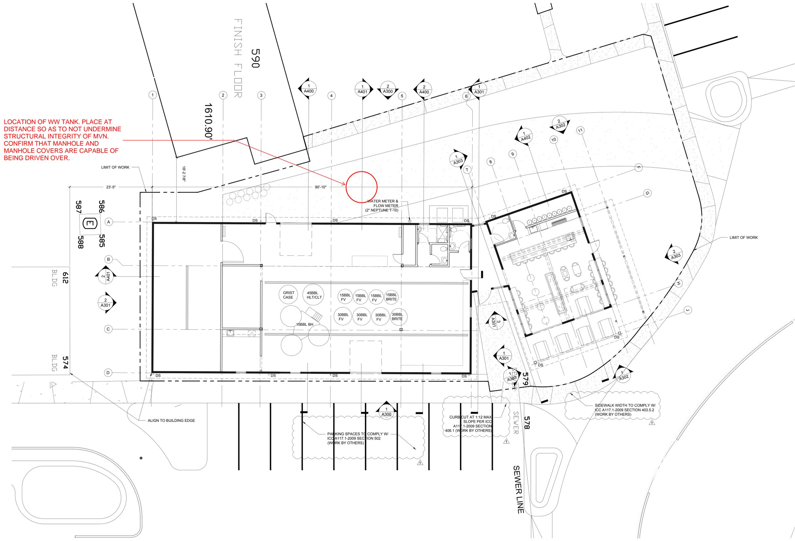
LOCATION OF WW TANK. PLACE AT DISTANCE SO AS TO NOT UNDERMINE STRUCTURAL INTEGRITY OF MVN. CONFIRM THAT MANHOLE AND MANHOLE COVERS ARE CAPABLE OF BEING DRIVEN OVER.
