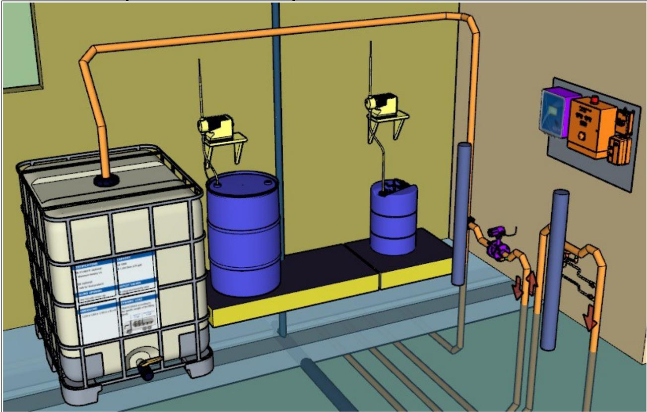
From left to right, we can see the calamity tank, chemical pumps and drums, flow meter loop, mixer loop, and controls. Here is a closer view of the controls and mixer loop:
