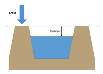
**<u>SET-BACK MEASUREMENTS</u>**---Measured from the top of bank, back to the point of discharge and/or crest of lagoon.
