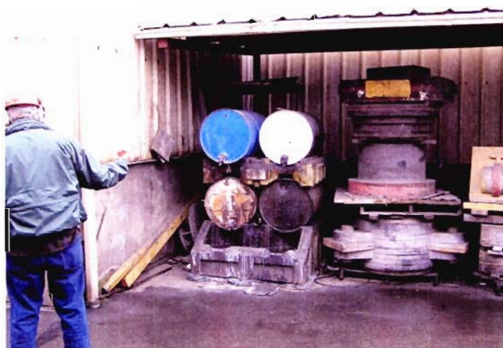
P2280419.JPG DESCRIPTION: ADEQUATE CHEMICAL HANDLING PROCEDURE; COVER, SECONDARY CONTAINMENT, AND DRIP PANS.
