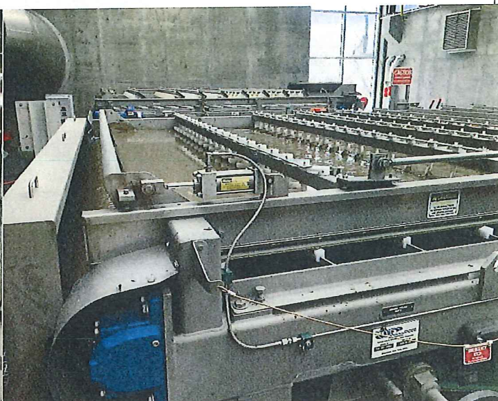
Photo # 30 Image: IMG_0143 Date: 6/25/2019 Taken by: Shawn McKone Description: Discharge end of GBT
