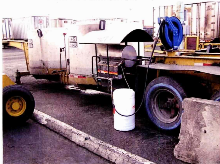
PC050100.JPG DESCRIPTION: FRESH WATER AND PRESSURE WASHER STORED ON A TRAILER OUTSIDE OF WASHING PAD CONTAINMENT. NOTICE OILY RESIDUE ON TRAILER AND THE GROUND BELOW, AS WELL AS A LEAK.
