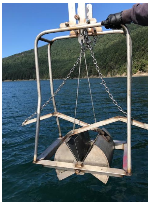
Figure 2. Left: Full sized ponar sampler with weights. Right: Custom-built stainless-steel Van Veen style grab sampler and frame used in this 2019 survey after the full-sized Ponar grab sampler was damaged during sampling.
