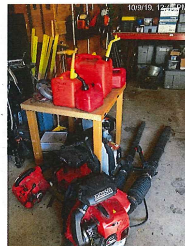
04 DESCRIPTION: NO SECONDARY CONTAINMENT FOR FUEL
