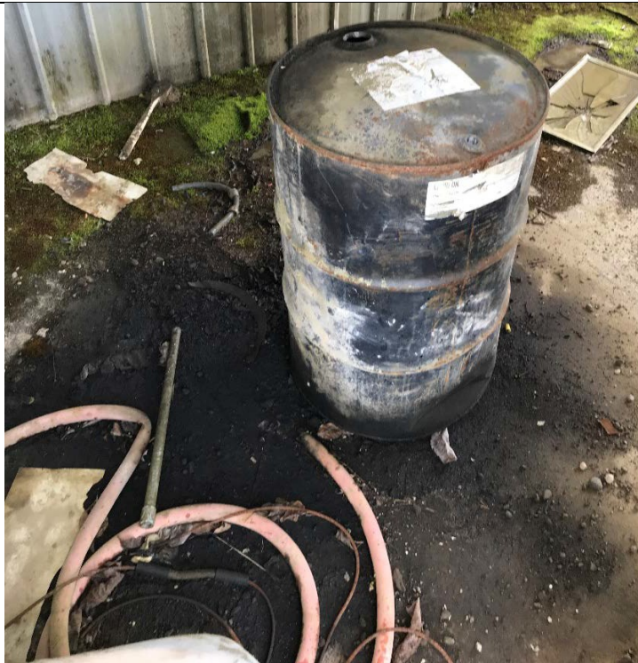
Photograph 4: Leaking drum labeled as chain oil, not in secondary containment.
