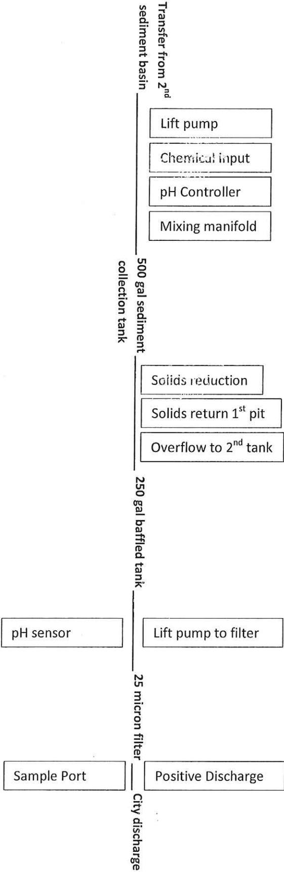
Attachment C. 2 Wash rack flow schematic for NC Machinery
