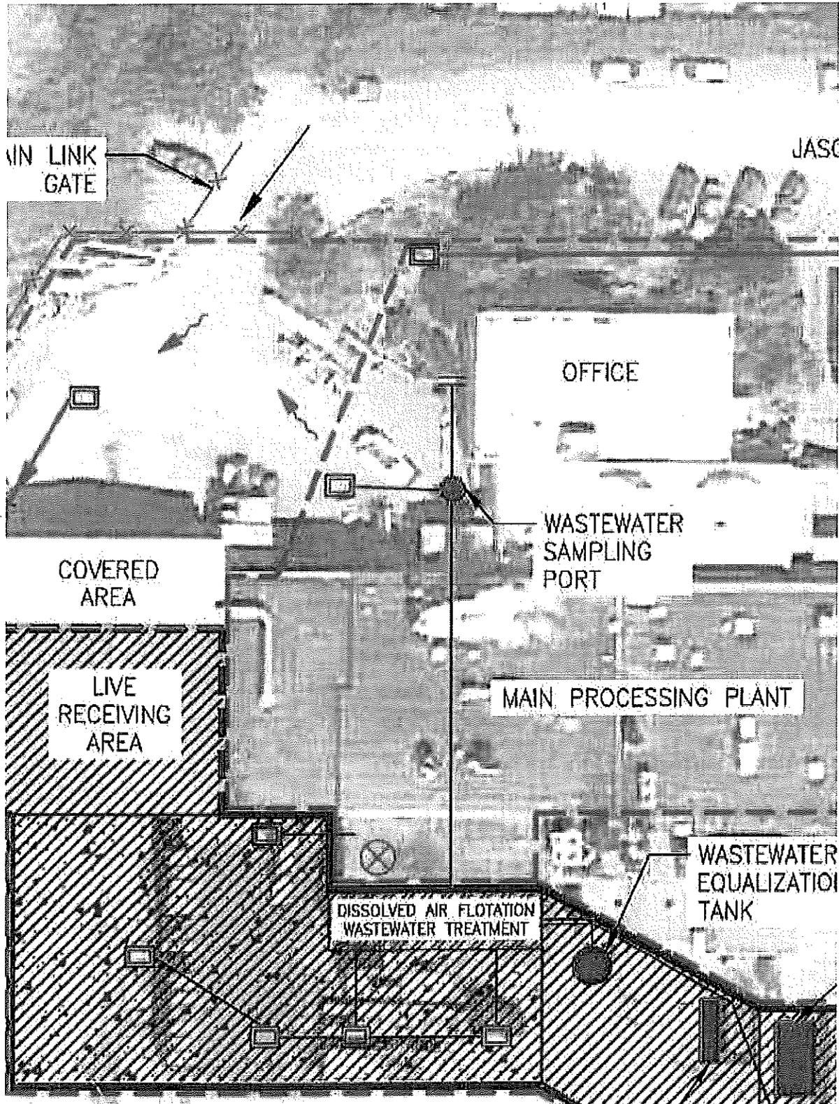
PROPOSED IMPROVEMENTS TO THE EXISTING WASTEWATER TREATMENT SYSTEM WILL OCCUR UP STREAM OF THE WASTEWATER SAMPLING PORT. IMPROVEMENTS ARE DESCRIBED IN ATTACHMENT C.4
