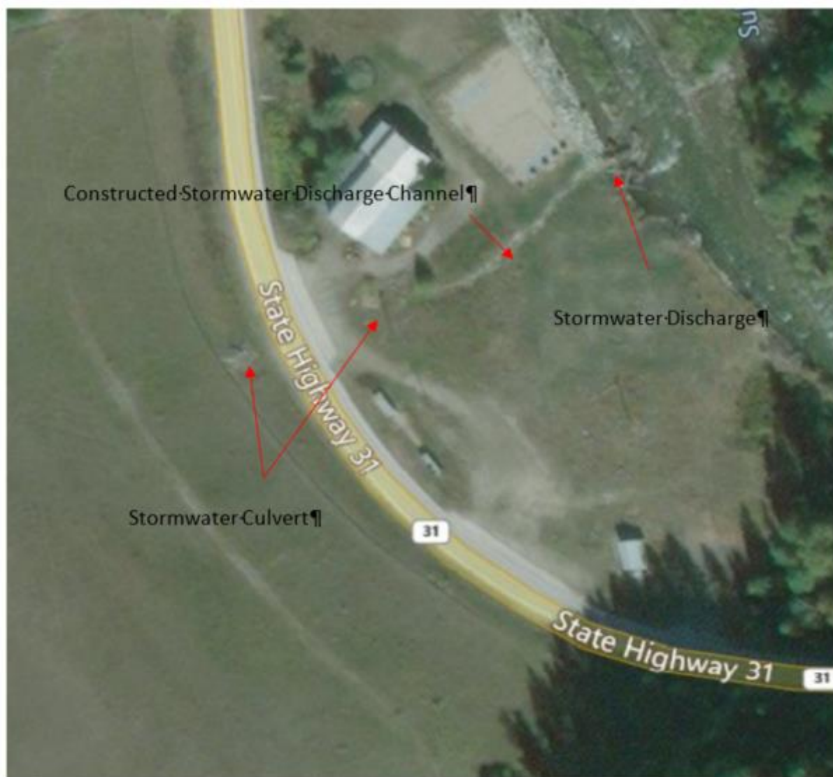
Figure 6: Closed CKD Pile Stormwater Drainage and Discharge
