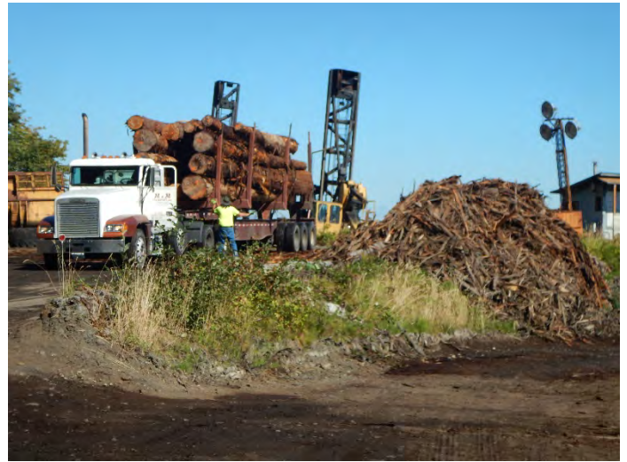
Photo #:20 (DSCN0419) Description: Facing northwest, photo of load cleaning process, where the logs are stripped of loose bark to reduce litter during transfer process. The discarded bark is left in the large pile on the right.
