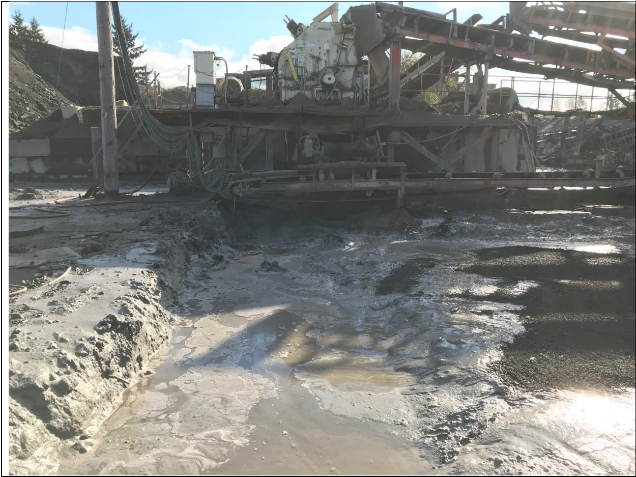
Photogrpah 2: Earthen basin next to the concrete crusher has a discharge groundwater with pH 12.17 measured (location 47.16498, -122.47294).
