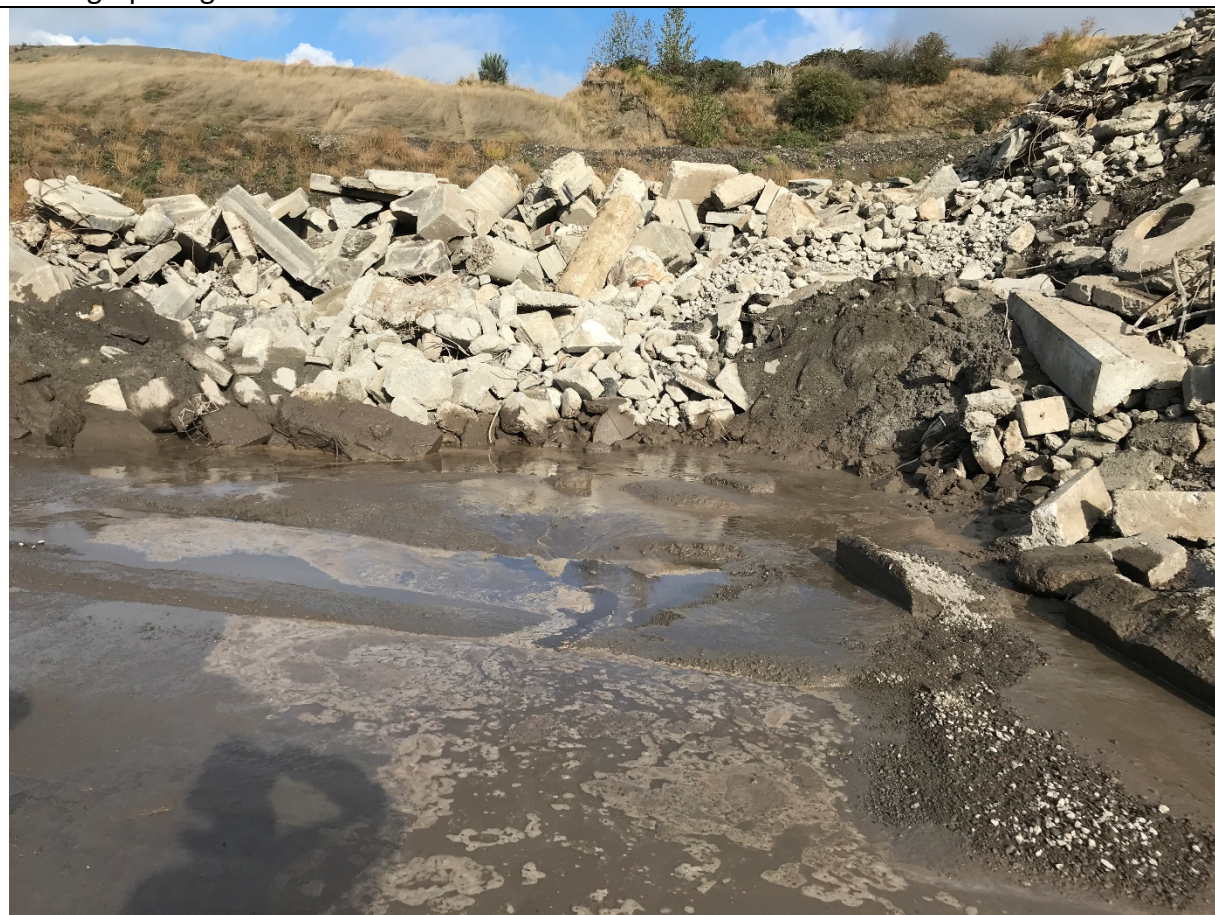
Photograph 1: Concrete stockpile pond discharge to groundwater with pH 12.30 (location 47.16558, -122.47318).
