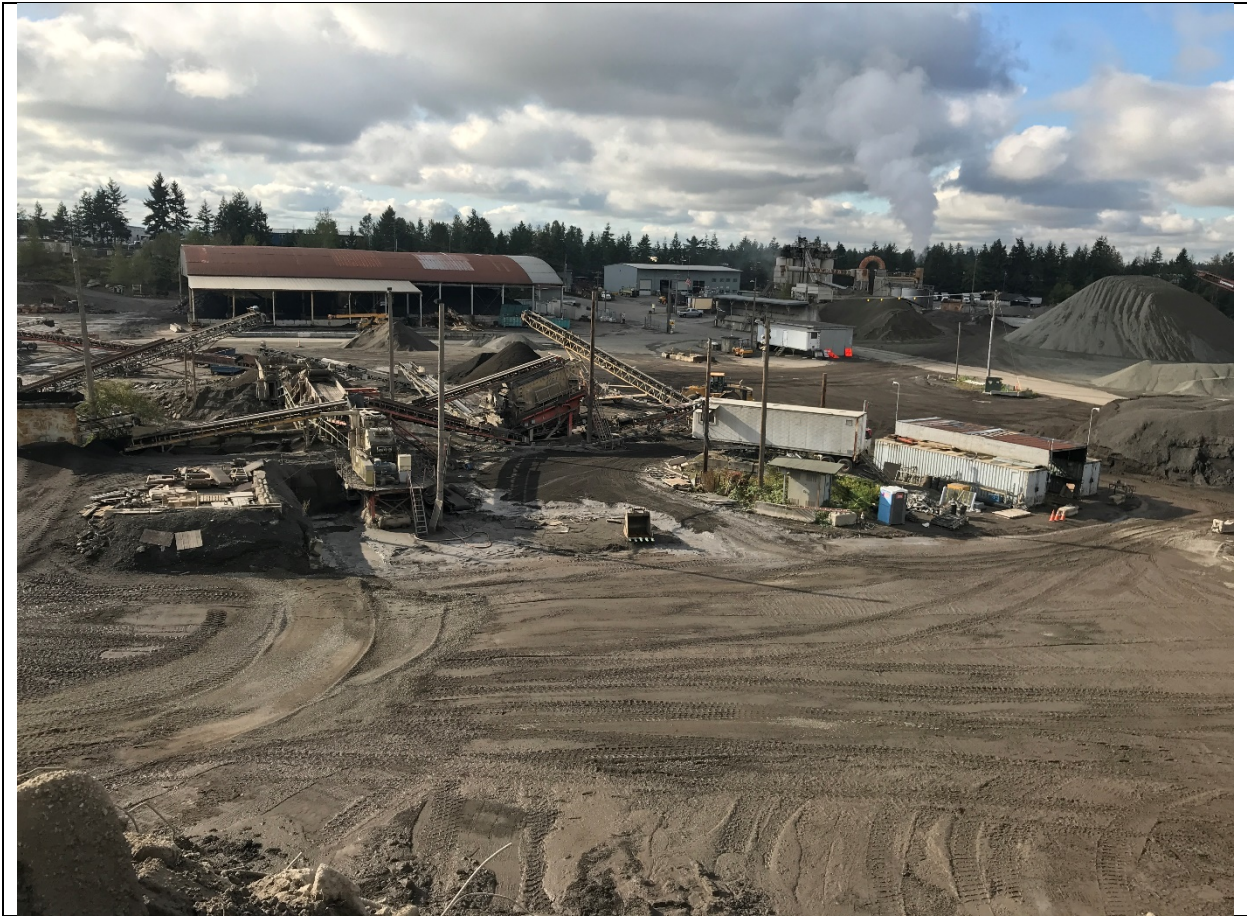
Photograph 5: Overview of concrete crushing storage or transfer of solid raw materials, by-products or finished products as seen from the top of the concrete stockpile.
