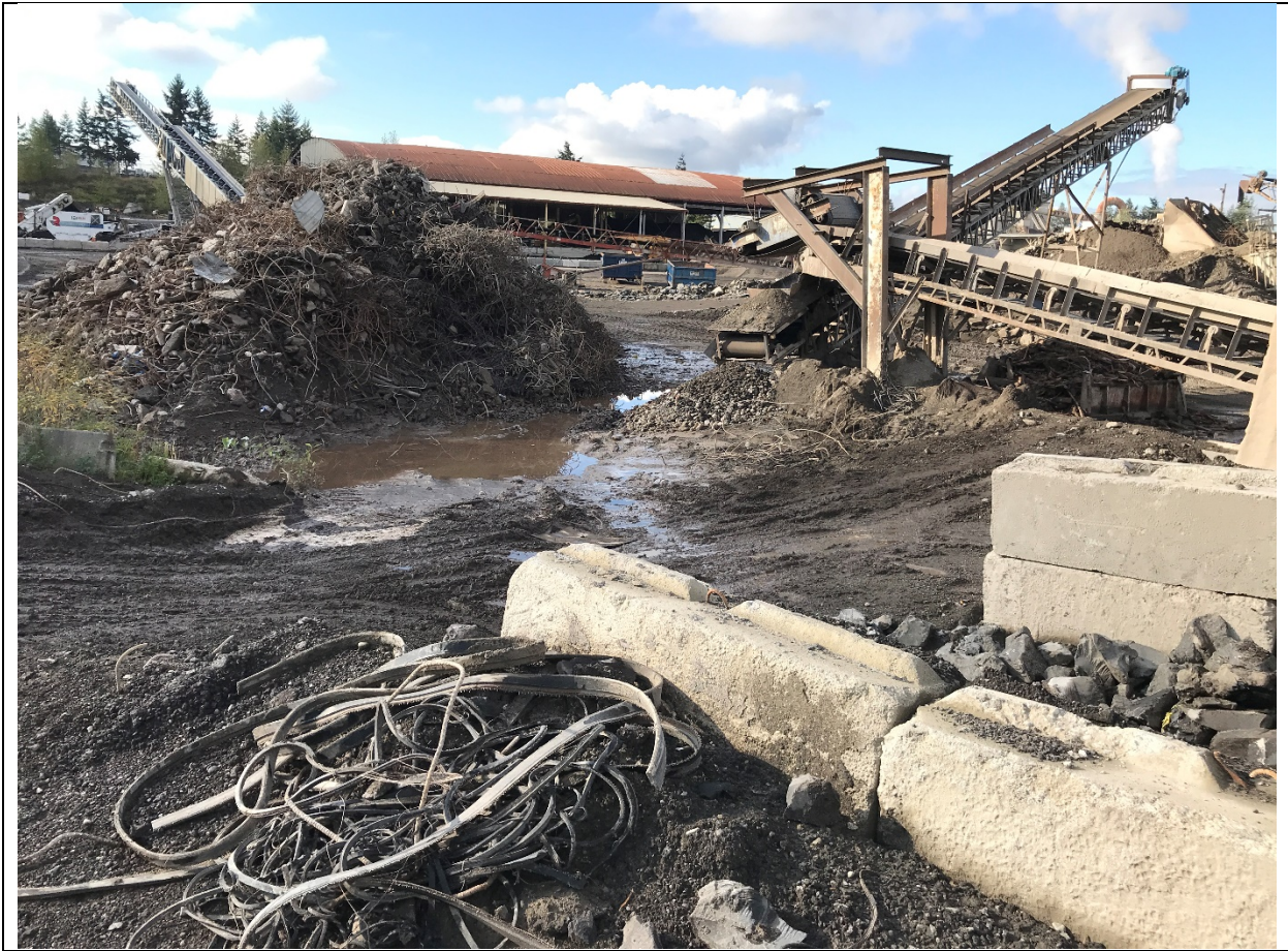
Photograph 4: Stormwater collection and ponding near the concrete recycling hopper discharges to groundwater with pH 10.16 measured (location 47.16504, -122.47276).
