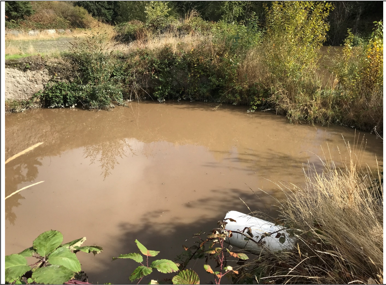
Photograph 5: Monitoring point location G002, approximately 950 feet from the concrete stockpile and crusher discharge points was not receiving piped stormwater during the inspection; pH 8.5 measured (location 47.16703, -122.47457).
