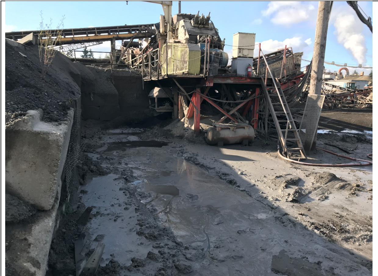
Photograph 3: Earthen basin filled concrete crushing by-product and stormwater discharge to groundwater.
