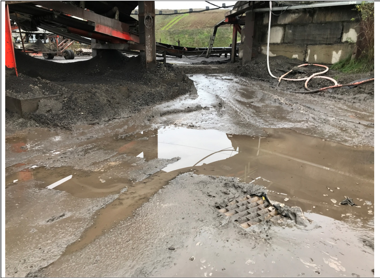
Photograph 3: Concrete recycling by-product sludge near a catch basin.
