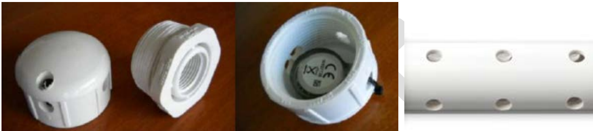
Figure 2. Examples of radiation shields (cap from RMRS, 2014) using an opaque color (avoid clear shields). Drill holes to facilitate water circulation.
