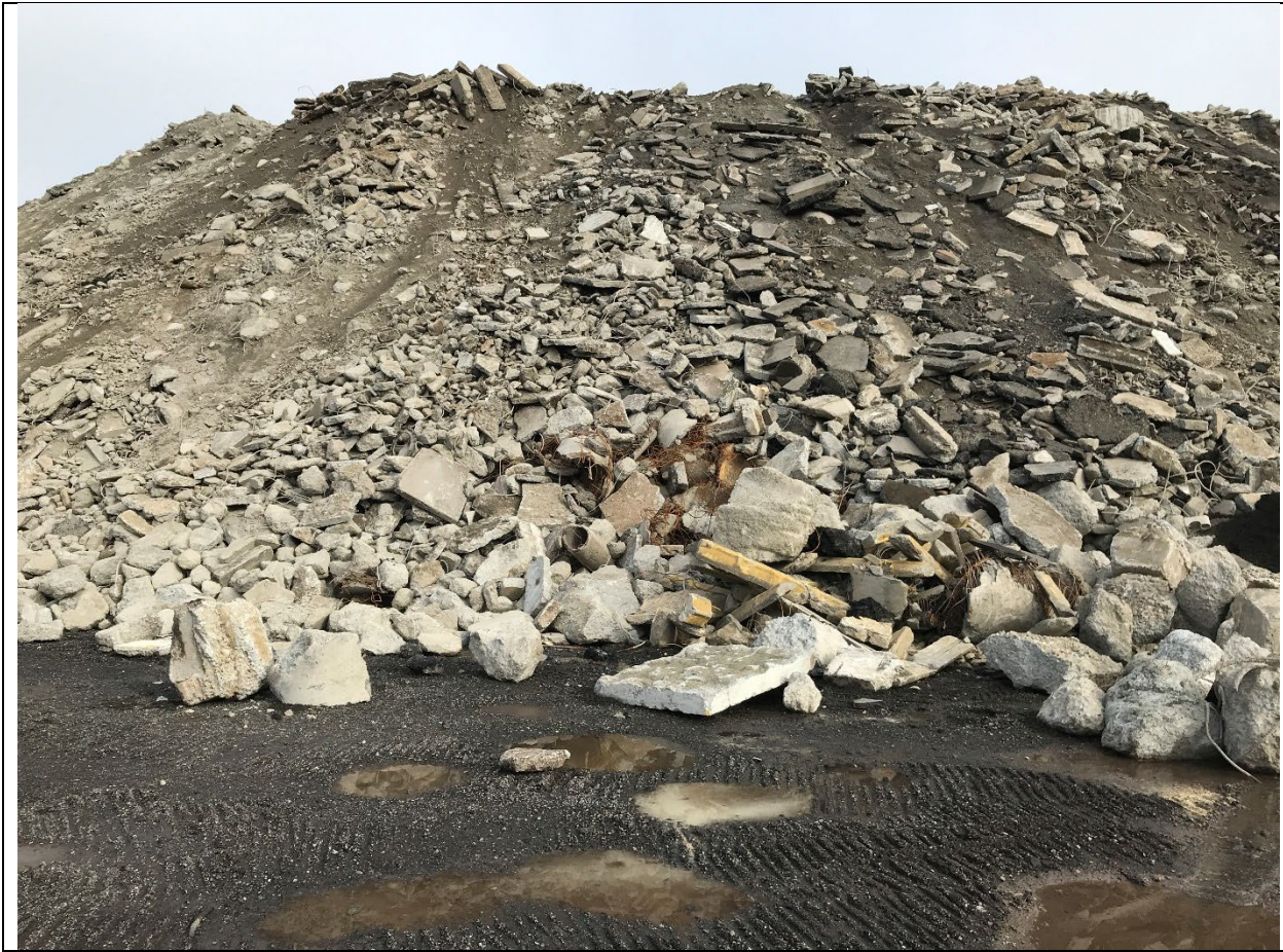
Photograph 3: Discharge to groundwater with concrete leachate below the concrete stockpile (monitoring point G003). The pH measured to 10.61 S.U. with a digital meter calibrated on January 25, 2022.
