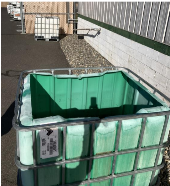
FIGURE 3: EVAPORATION TOTES FOR MINT OIL WATER IMPURITIES
