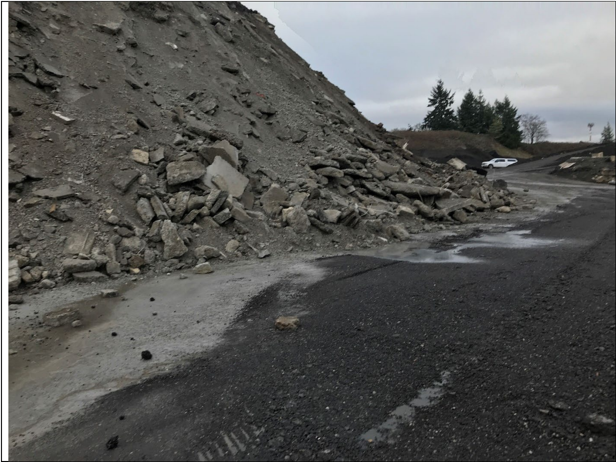
Photograph 3: Near the boundary of paved and unpaved areas where concrete pile runoff is draining towards the pavement.
