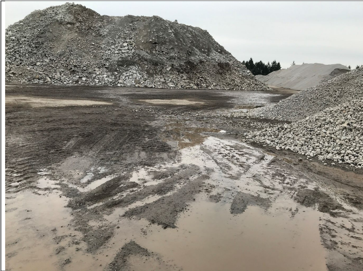
Photograph 3: Drainage path of the concrete crushing and stockpile area runoff. I measured a pH of 10.78 in pooling water on the bare ground.
