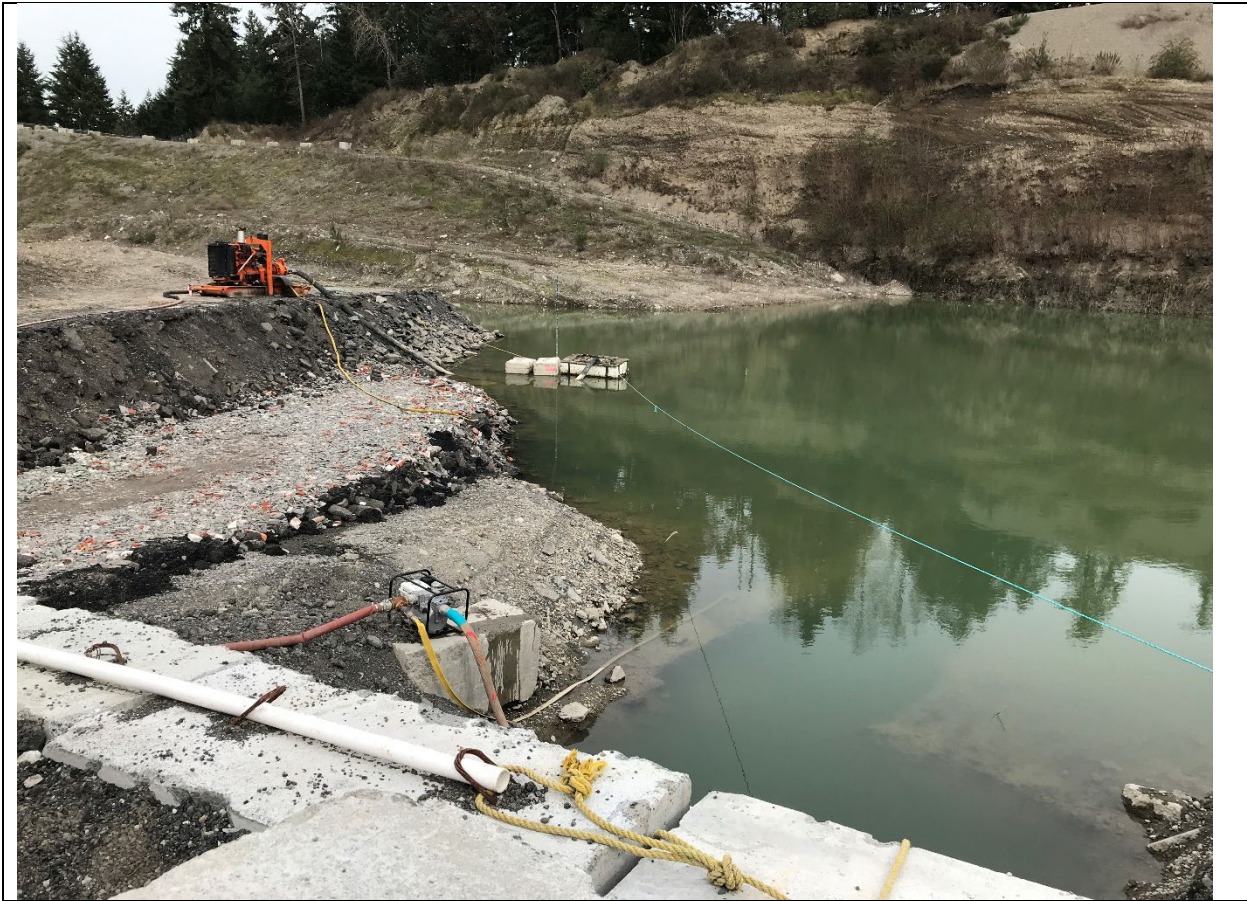
Photograph 5: Main infiltration pond - monitoring point SP2, I measured a pH of 9.07 S.U. The pump was not running and surface water discharge was not occurring during the inspection.
