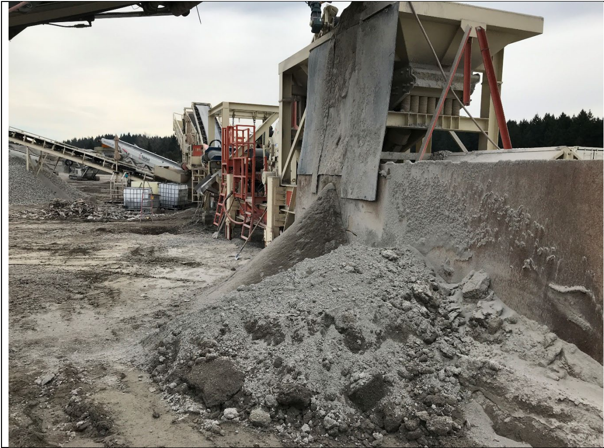
Photogrpah 2: Accumulation of concrete fines from the crusher and concrete recycling operations.
