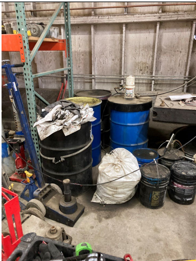
Photo 35 Description: Photo of drums and buckets without secondary containment.
