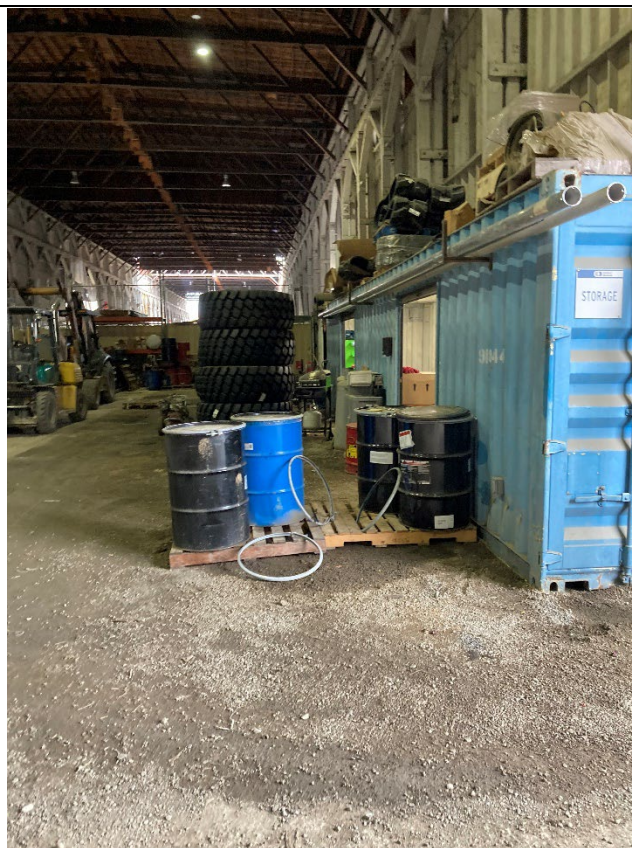
Photo 36 Description: Photo of drums without secondary containment.
