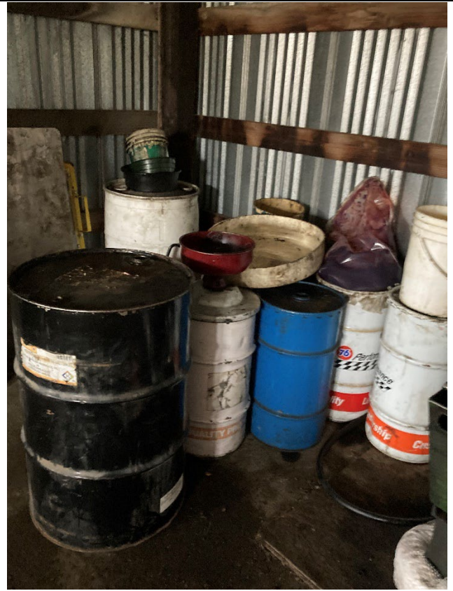
Photo 14 Description: Photo of drums without secondary containment.
