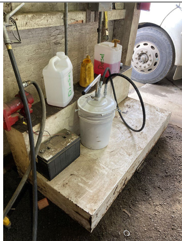
Photo 32 Description: Photo of containers with diesel without secondary containment.
