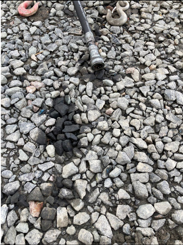
Photo 41 Description: Photo of black residue on ground; leaks observed coming out of hose.
