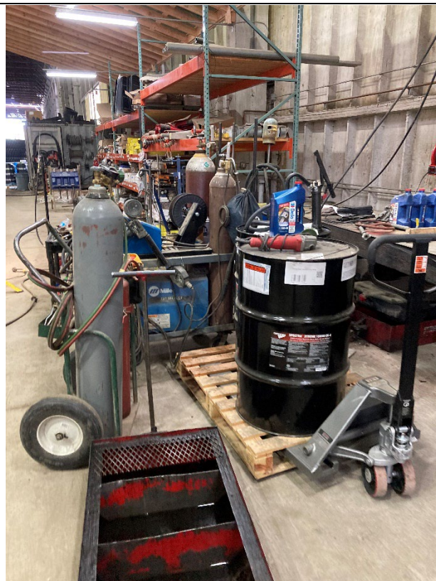
Photo 34 Description: Photo of drum without secondary containment.
