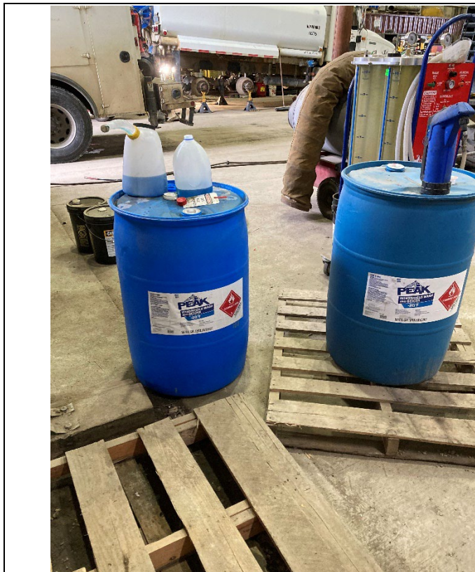
Photo 33 Description: Photo of drums without secondary containment.
