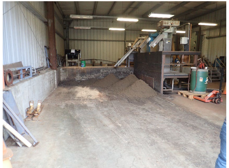
Photo No.12 Date: 8/23/21 taken by Madison Diaz Description: Sludge Dewatering System
