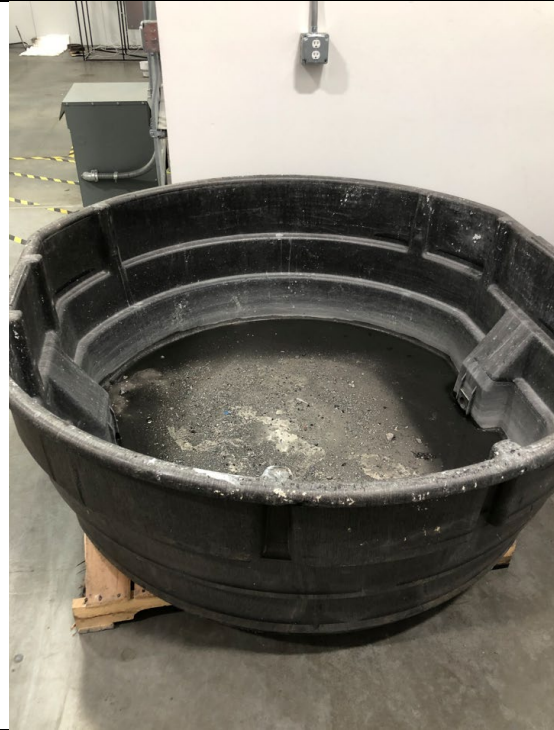
Photo 2: Tub used for washing molds after pattern burn out, note remaining accumulated ash at the bottom of the tub.
