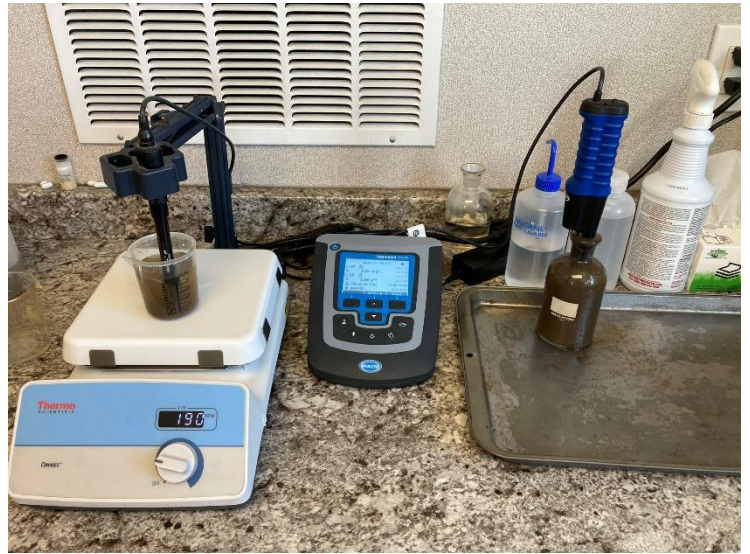
pH and DO grab sample: readings pH 6.88, DO 2.83 mg/L
