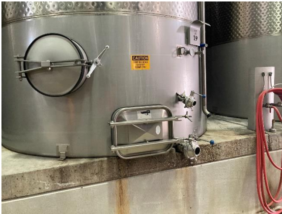
Production tank – high and low door for removing solids
