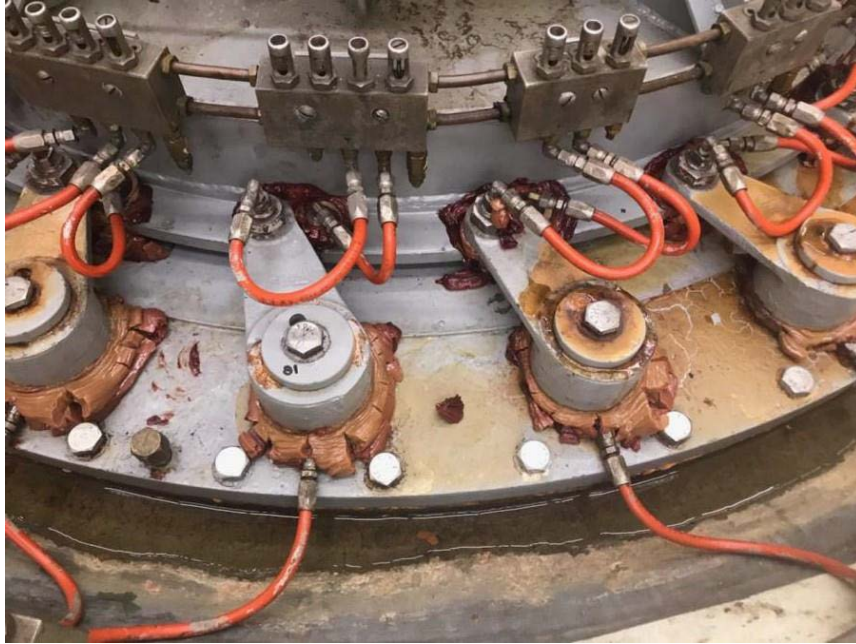
Figure 4 The complete penetration of the Panolin Biogrease EP2 in the Fish Attraction Water Pump #1, into the above water fittings for the wicket gates. The taupe brown colored grease can be seen covering the red colored grease.
