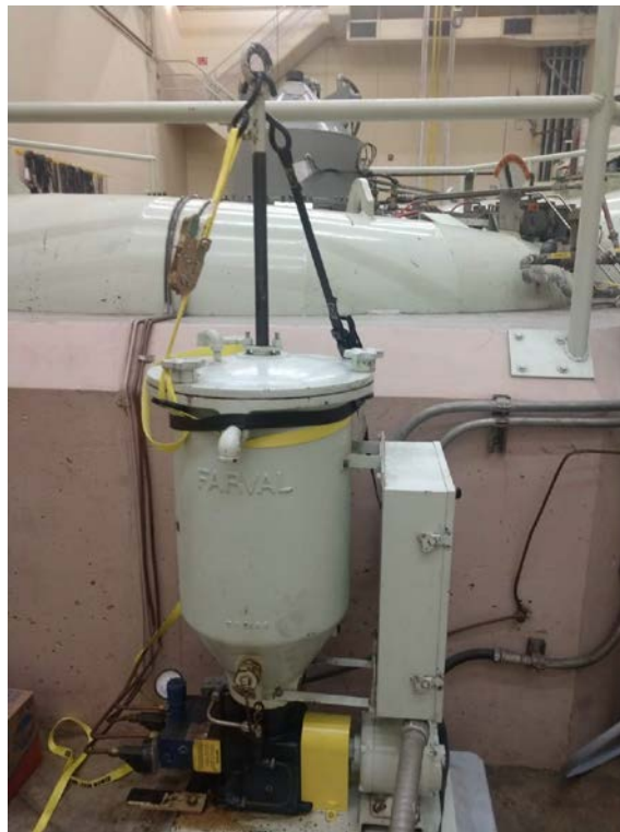
Figure 6 The temporary solution of strapping the plunger down to the reservoir, that was created to compensate for the thick viscosity of the BioBlend HDS2 EAL grease.
