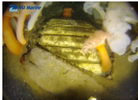
Figure 2: Typical anode bracelet condition
