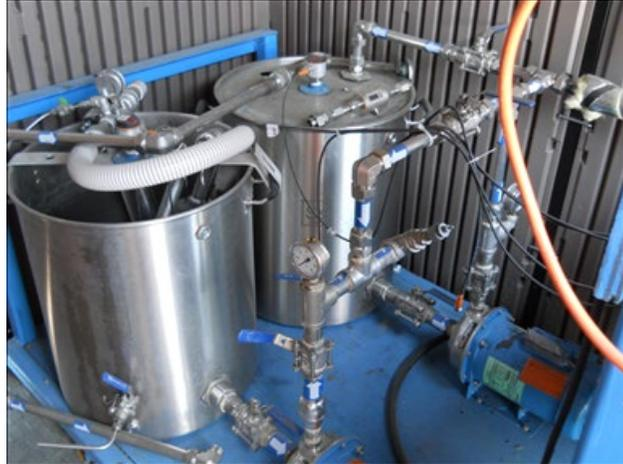
Photo 14: Walnut shell filtration system inlet wet well and pumps
