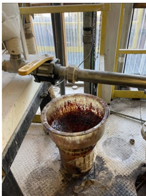
Photo 22. Catch for when samples are taken to test glue. Proper secondary containment?
