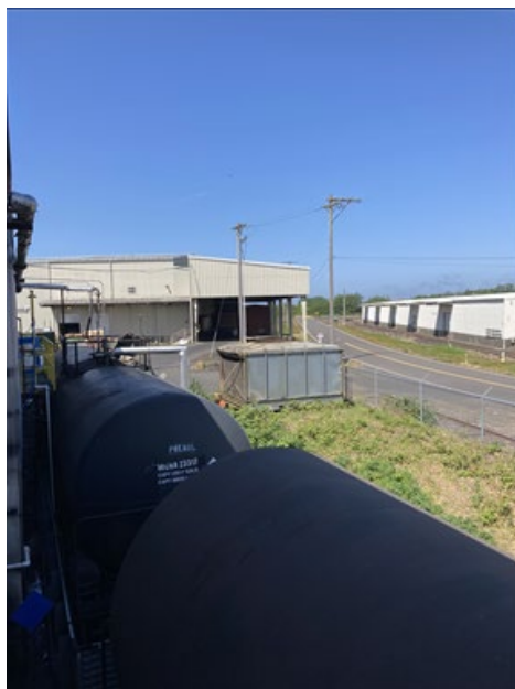
Photo 14. Rail cars holding phenol (foreground). Rented rail car in back, transfer rail car in front. Rectangular metal apparatus for cooling water (background).
