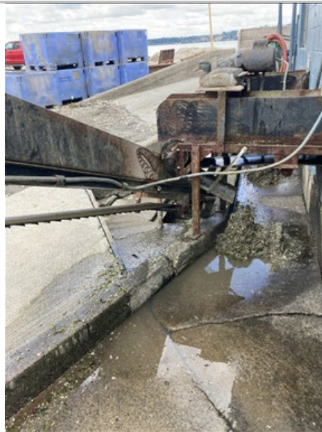
Photo 4. Outside catchment. Conveyer belt for solid waste
