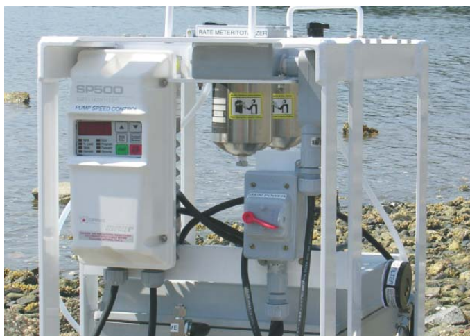
Figure 3. Infiltrax 300 sampler uses high-capacity filters and XAD-2 resin columns to extract PCBs, PBDE, and dioxins/furans from large volumes of sample water.
