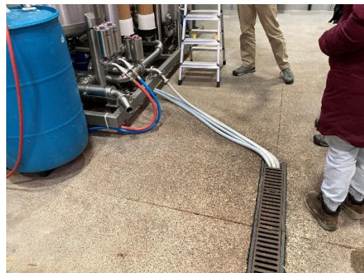
Oenoflow hose going to floor drain
