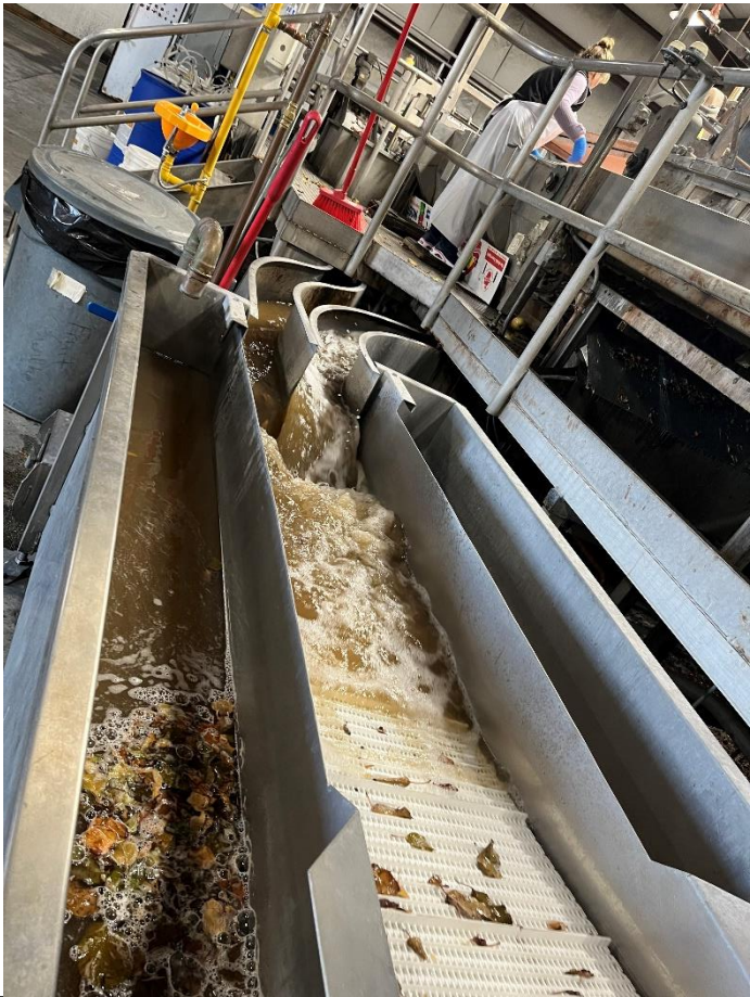
Photo 2 Description: Float water being filtered from leaves and debris that comes in with the fruit. Debris is collected and disposed of as solid waste.
