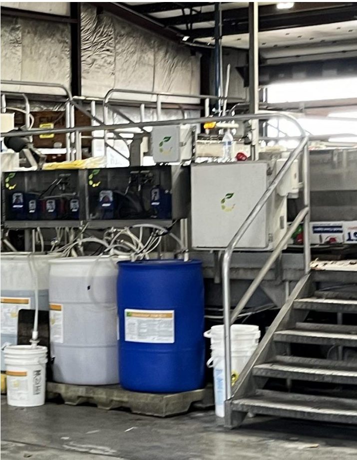
Photo 4 Description: chemical usage on the line for fruit cleaning, disinfection, and polishing (aesthetics)
